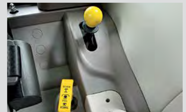
Easy mechanical PTO speed engagement.
