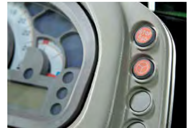
Stop and Go activation via push button.
