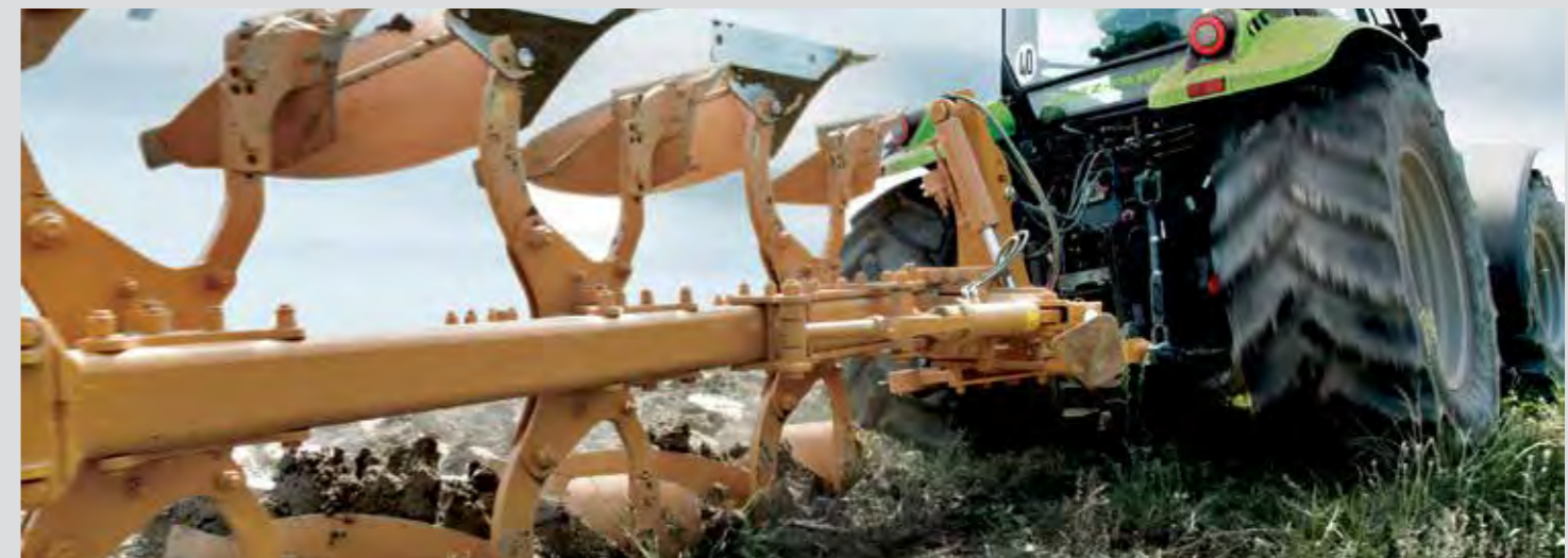
Heavy duty category 2 three point linkage.
