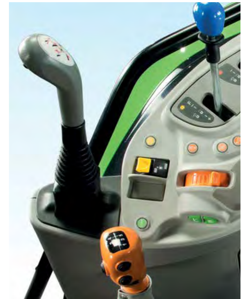
The loader control joystick integrates perfectly in the right-hand console.
