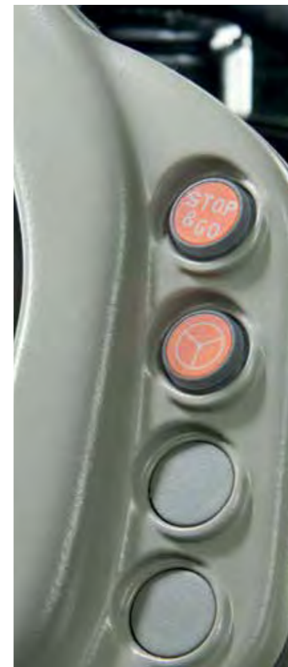
Pushbuttons to activate the Stop&Go and SDD functions.
