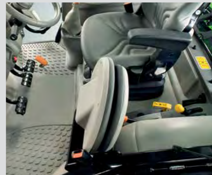
New position and shape for the passenger seat with hinged lower pad.
