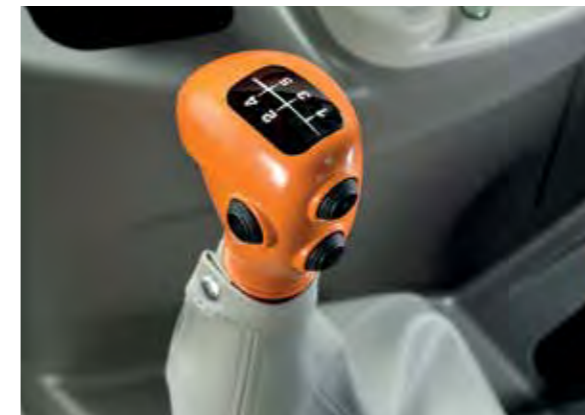
The gear lever with Powershift speed change buttons and the ComfortClutch electro-hydraulic clutch button.
